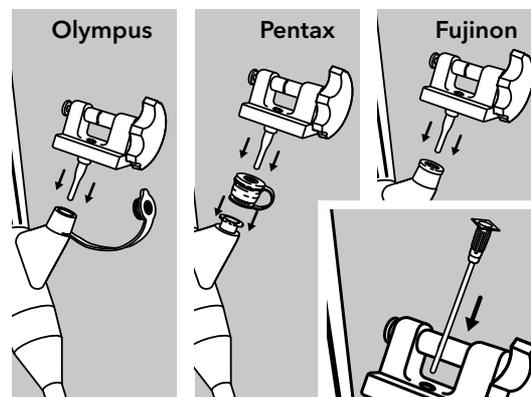
Insert the ligator handle into the endoscope accessory channel.
