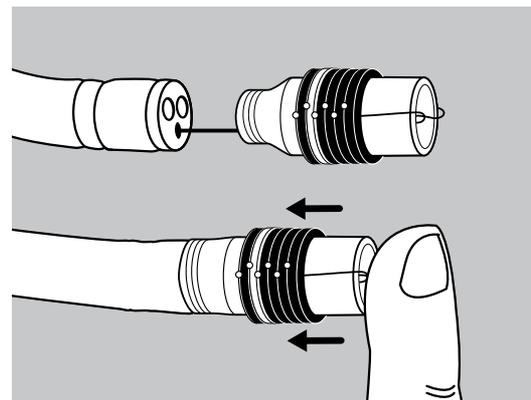
Secure the friction fit adapter of the barrel to the tip of the endoscope and advance the barrel as far as possible.
